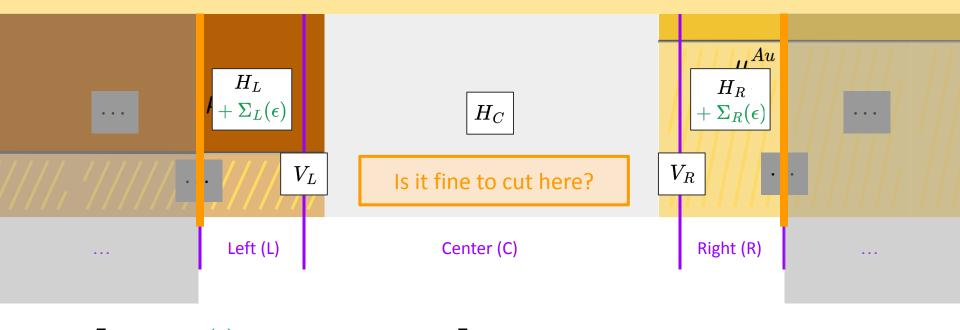
$$H = egin{bmatrix} H_L + oldsymbol{\Sigma}_L(\epsilon) & V_L & 0 \ V_L^\dagger & H_C & V_R \ 0 & V_R^\dagger & H_R + oldsymbol{\Sigma}_R(\epsilon) \end{bmatrix}$$
