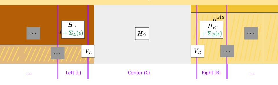
$$H = egin{bmatrix} H_L + oldsymbol{\Sigma}_L(\epsilon) & V_L & 0 \ V_L^\dagger & H_C & V_R \ 0 & V_R^\dagger & H_R + oldsymbol{\Sigma}_R(\epsilon) \end{bmatrix}$$
